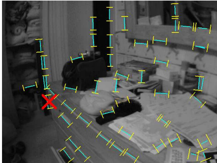
Figure 5.3: An example of outlier detection performed by the robust data association algorithm
