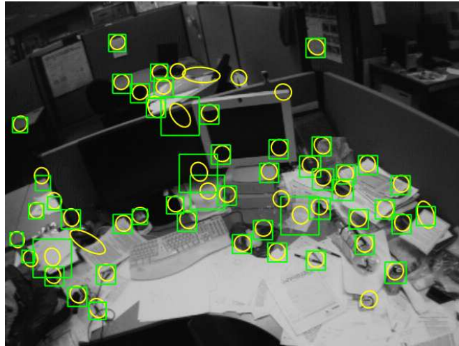
Figure 6.2: Active search regions for a frame from a desktop sequence. The search ellipses are yellow, and successful observations are shown with green boxes. The observations are of different scales in the image because of their distinct warps for the current pose
