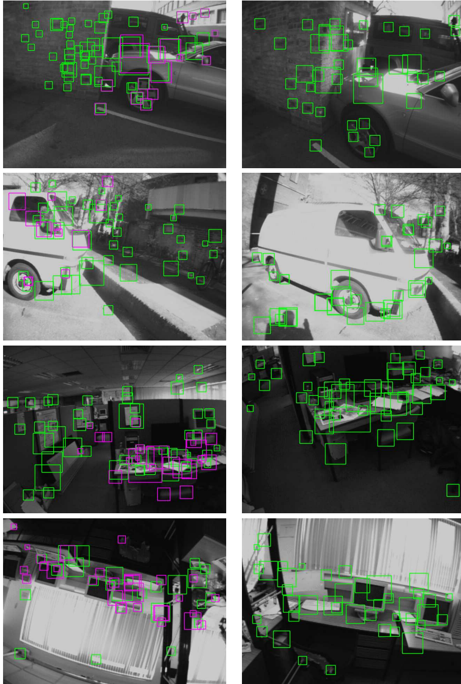
Figure 7.3: Left: video frames of loop closure or recovery events. Right: the most similar previous view of the scene. Normal observations are green, while observations via candidate edges are magenta
